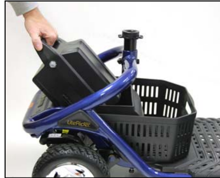
Figure 21. Battery Pack Installation
