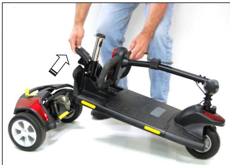
Figure 17. Separating the Drivetrain and Frame
