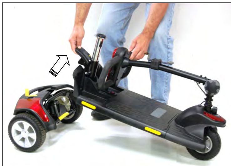
Figure 17. Separating the Drivetrain and Frame
