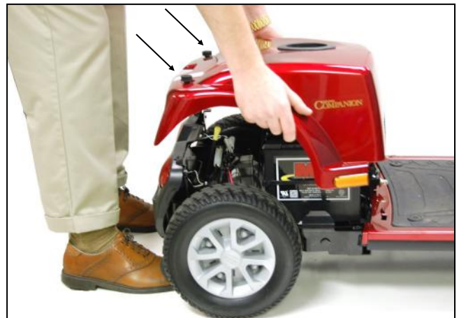
FIGURE 16. REMOVING THE REAR SHROUD
