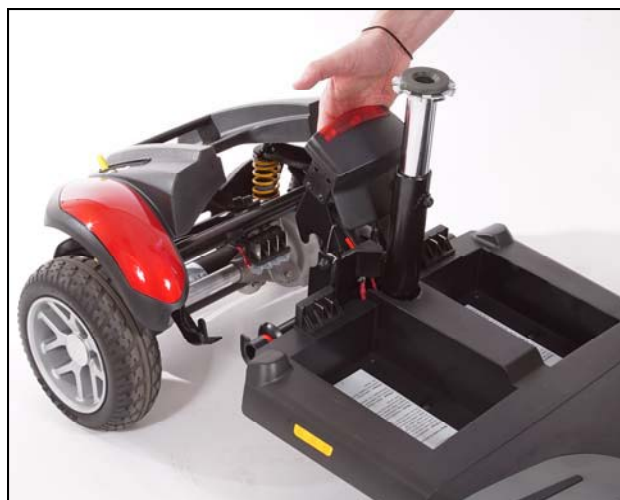
Figure 17. Separating the Drivetrain and Frame
