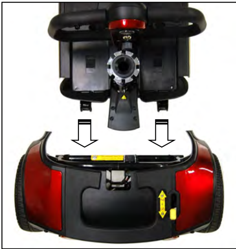
Figure 19. Drivetrain Alignment
