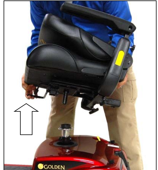
FIGURE 14. REMOVING THE SEAT
