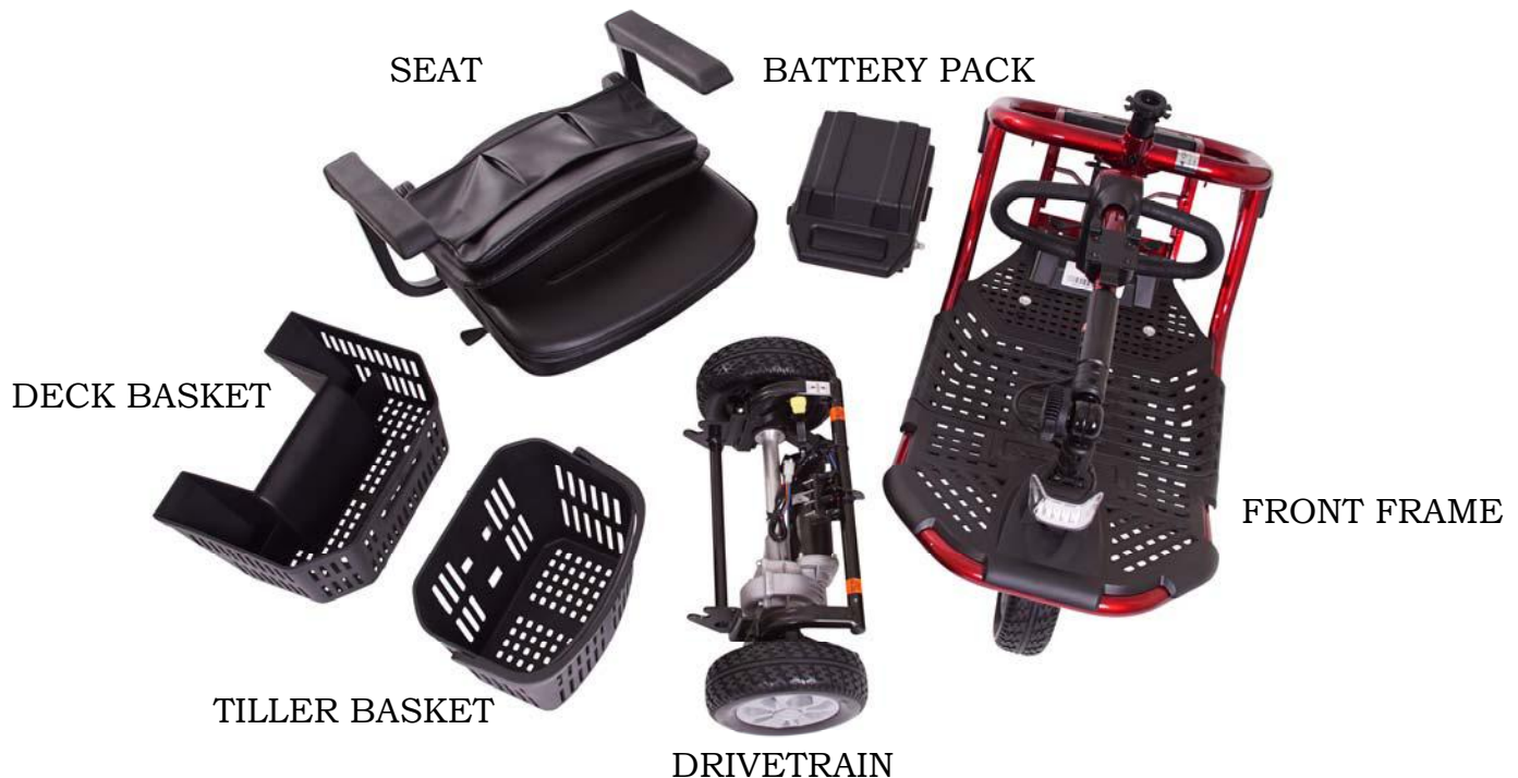
Figure 19. LiteRider Components (3-wheel)
