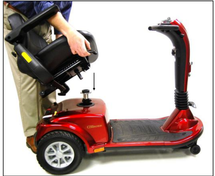
FIGURE 24. REINSTALL THE SEAT
