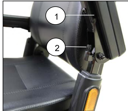
Figure 9. Armrest Angle Adjustment
