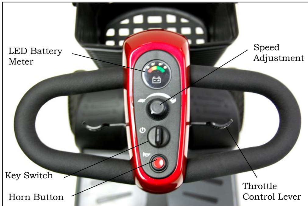
Figure 5. Buzzaround XL™ Delta Tiller Control Panel
