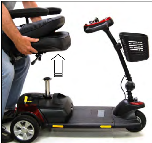
Figure 14. Removing the Seat
