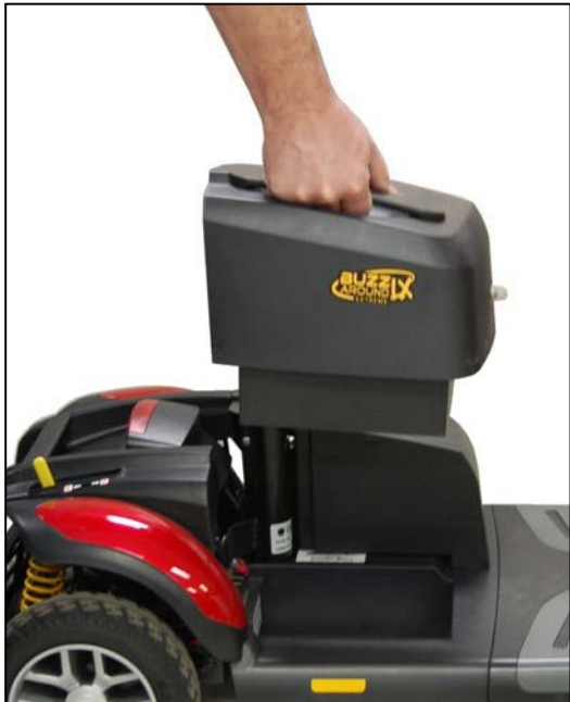
Figure 23. Battery Pack Installation
