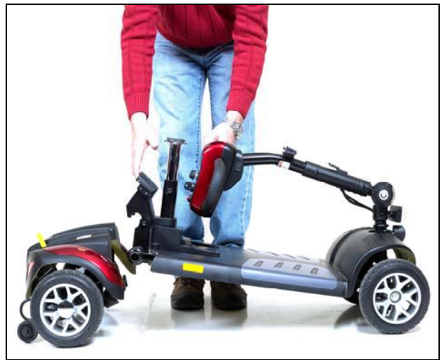
Figure 20. Connecting Frame and Drivetrain
