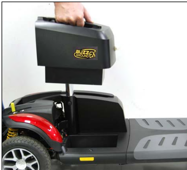
Figure 21. Battery Pack Installation
