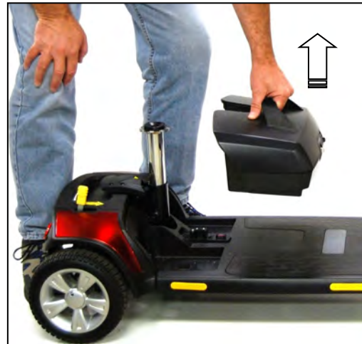
Figure 15. Removing the Battery Pack
