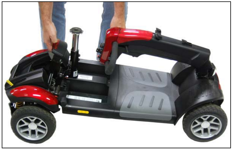
Figure 22. Connecting Frame and Drivetrain
