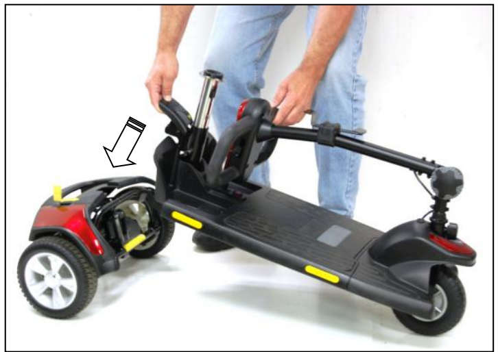
Figure 20. Connecting Frame and Drivetrain
