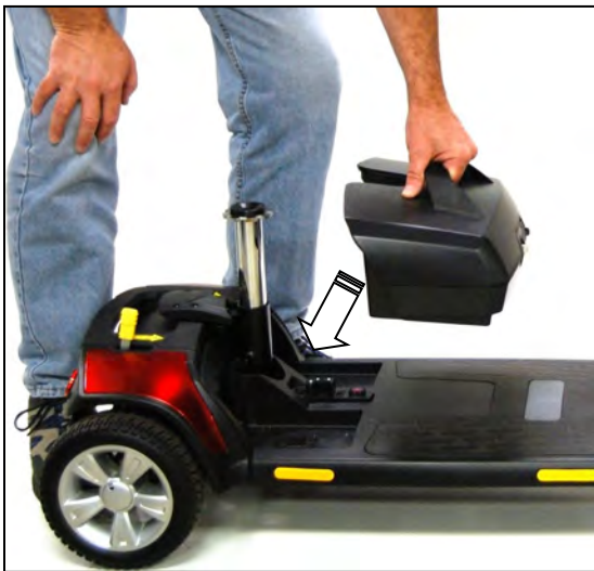
Figure 21. Battery Pack Installation
