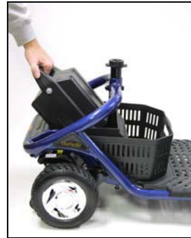
Figure 14. Removing the Battery Pack
