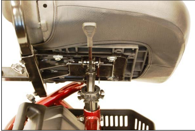
Figure 23. Installing the Seat
