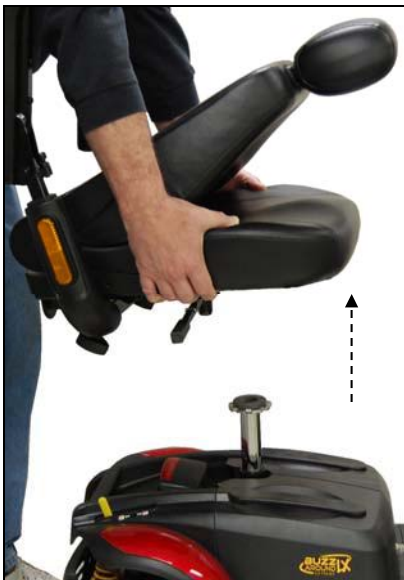
Figure 16. Removing the Seat
