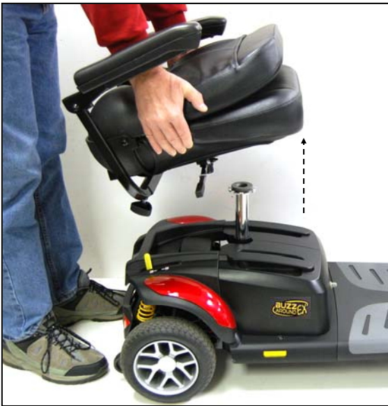
Figure 14. Removing the Seat
