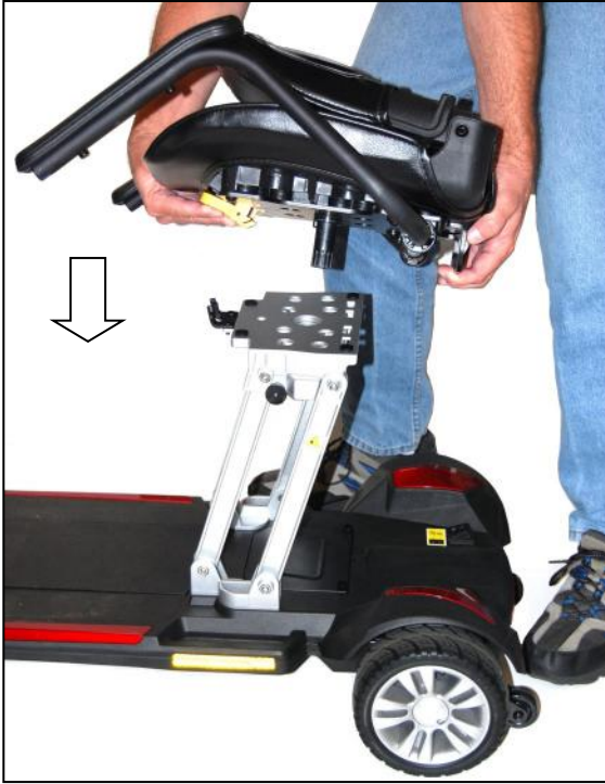
Figure 21. Installing Seat
