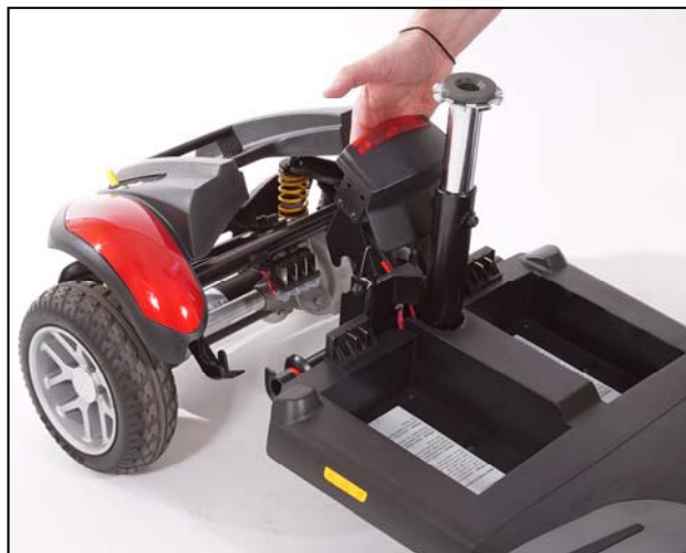
Figure 19. Separating the Drivetrain and Frame
