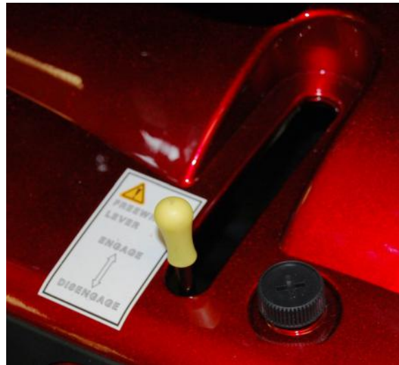
FIGURE 12. FREEWHEEL LEVER (DISENGAGED)
