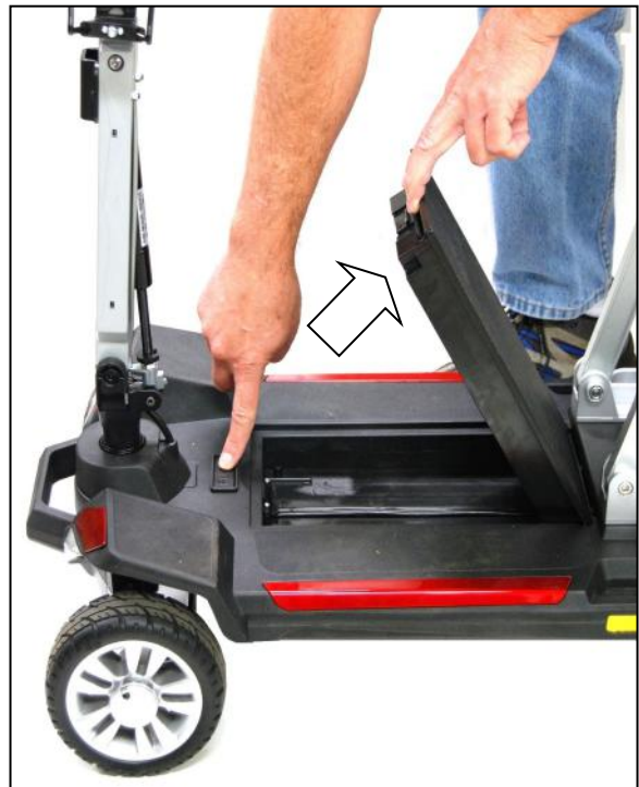
Figure 13. Removing Battery Pack
