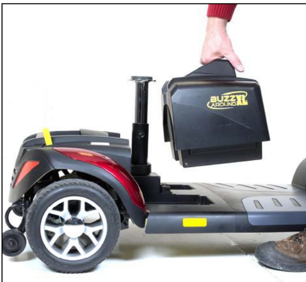
Figure 21. Battery Pack Installation
