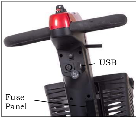
Figure 6. 1 AMP USB Charging Port
