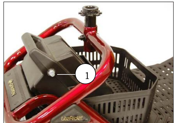
Figure 27. Main Circuit Breaker
