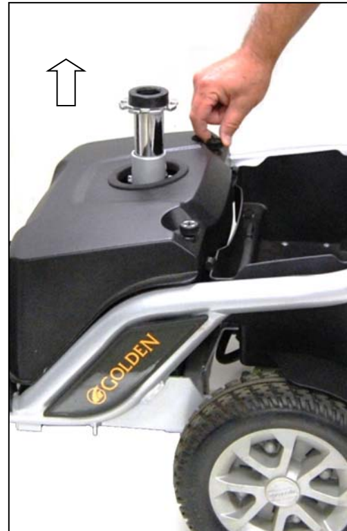
Figure 14. Removing the Battery Cover
