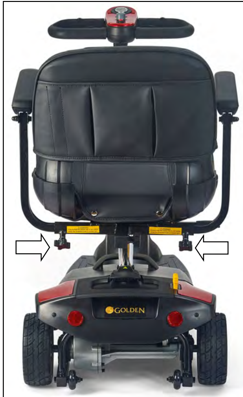
Figure 6. Armrest Width Adjustment
