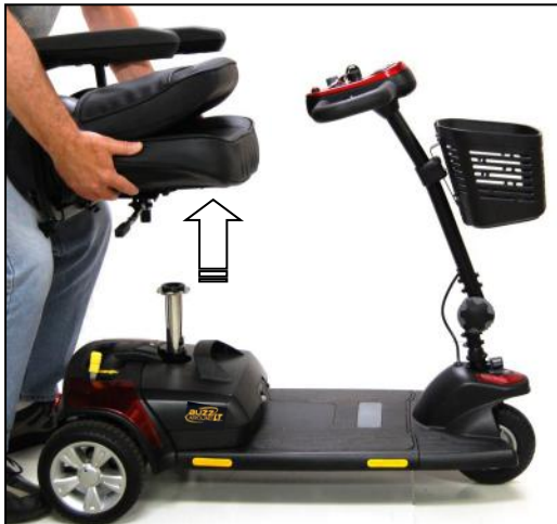
Figure 14. Removing the Seat
