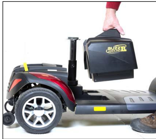
Figure 15. Removing the Battery Pack
