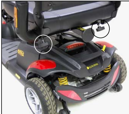
Figure 8. Armrest Width Adjustment
