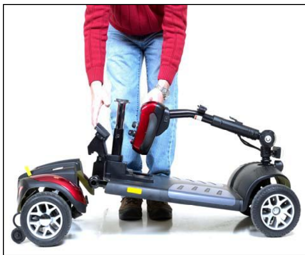
Figure 20. Connecting Frame and Drivetrain
