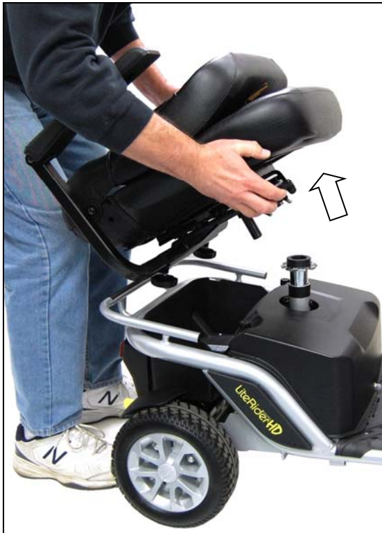
Figure 13. Removing the Seat
