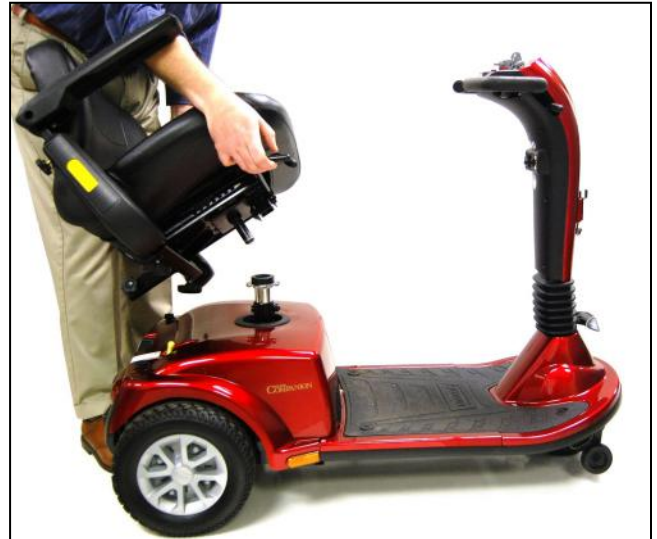
FIGURE 15. REMOVING THE SEAT
