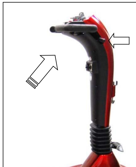
FIGURE 19. RAISE THE TILLER
