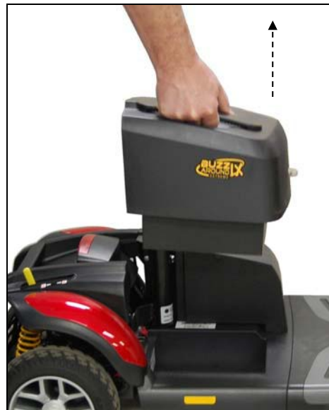
Figure 17. Removing the Battery Pack
