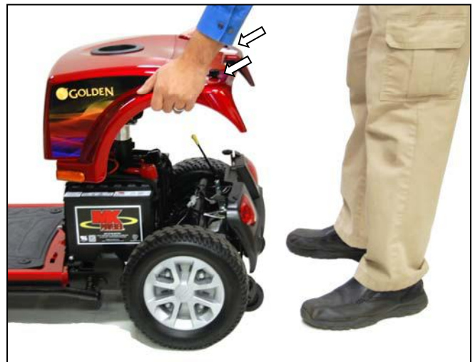
FIGURE 15. REMOVING THE REAR SHROUD
