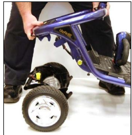
Figure 18. Lifting the Frame
