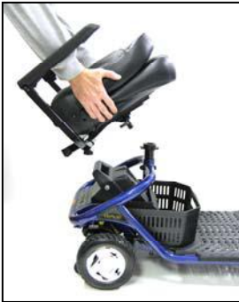
Figure 13. Removing the Seat
