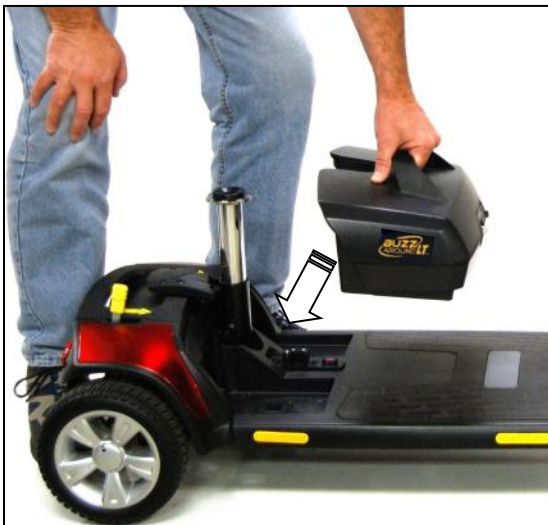
Figure 21. Battery Pack Installation
