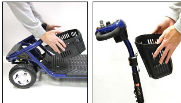
Figure 15. Removing the Baskets
