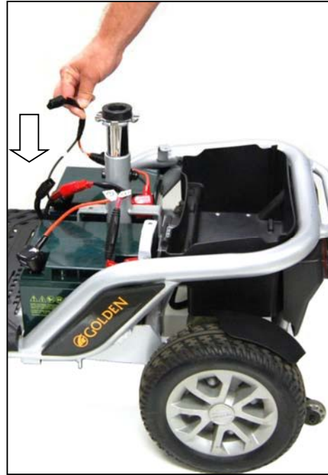
Figure 21. Installing the Batteries
