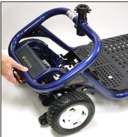
Figure 17. Releasing the Drivetrain
