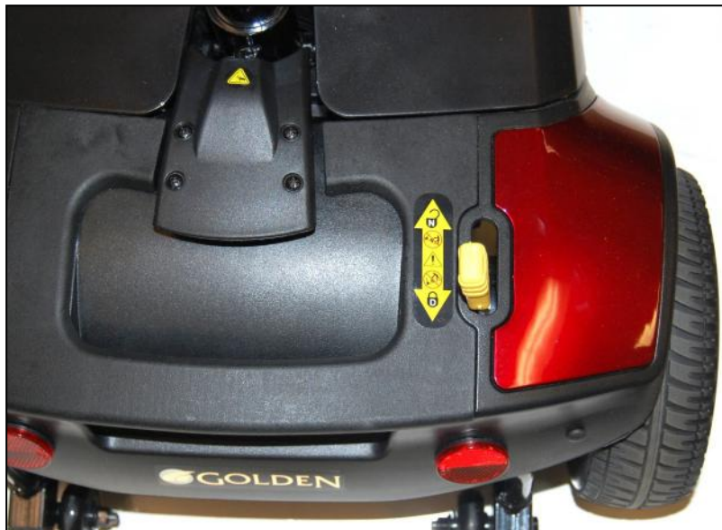
Figure 11: Freewheel Lever (Drive Position)
