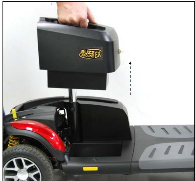
Figure 15. Removing the Battery Pack
