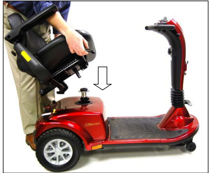
FIGURE 22. REINSTALL THE SEAT
