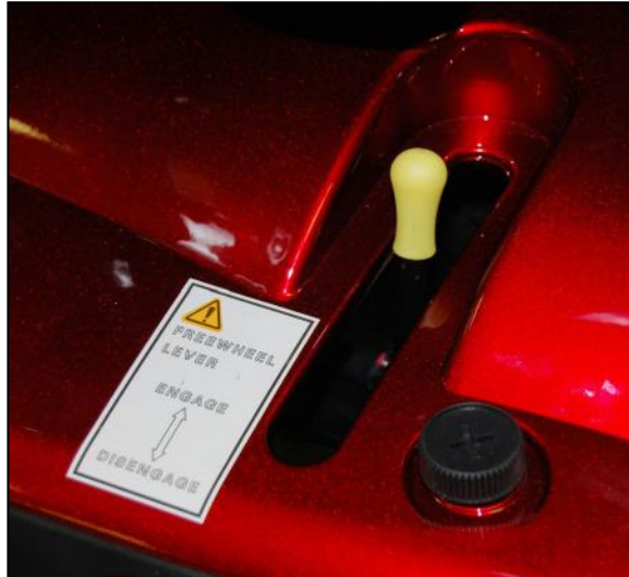
FIGURE 11. FREEWHEEL LEVER (ENGAGED)
