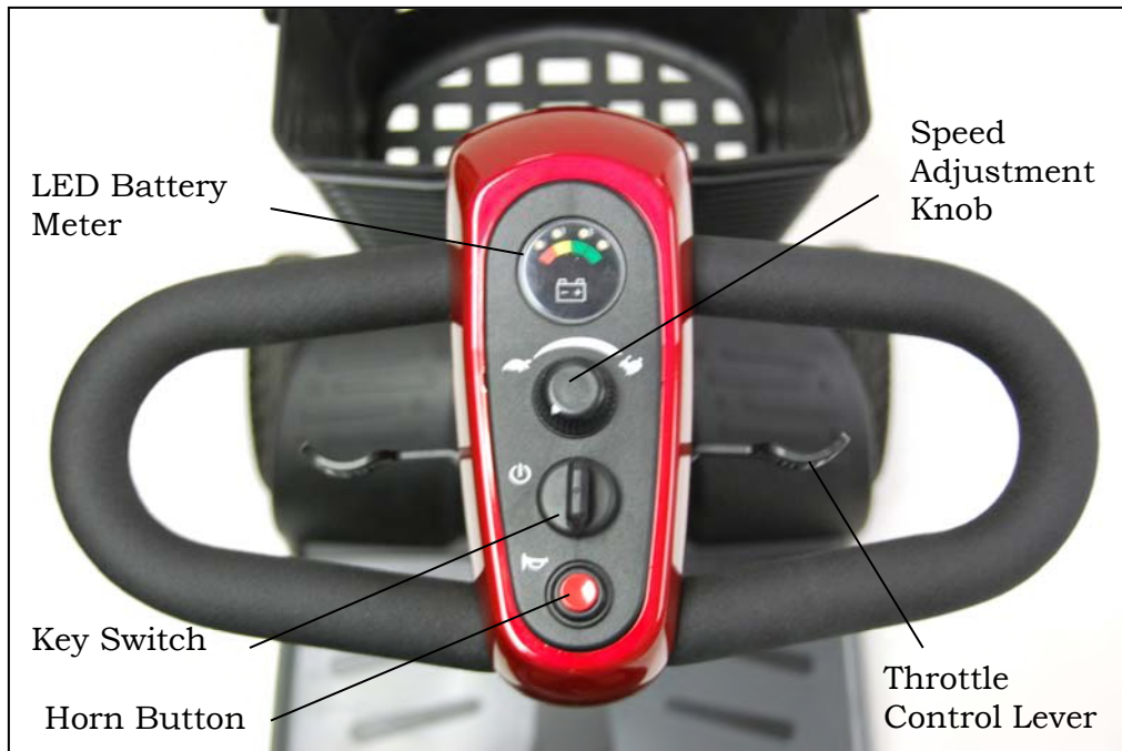
Figure 5. Buzzaround Luxury™ Delta Tiller Control Panel
