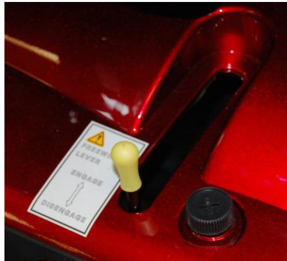
FIGURE 12. FREEWHEEL LEVER (DISENGAGED)
