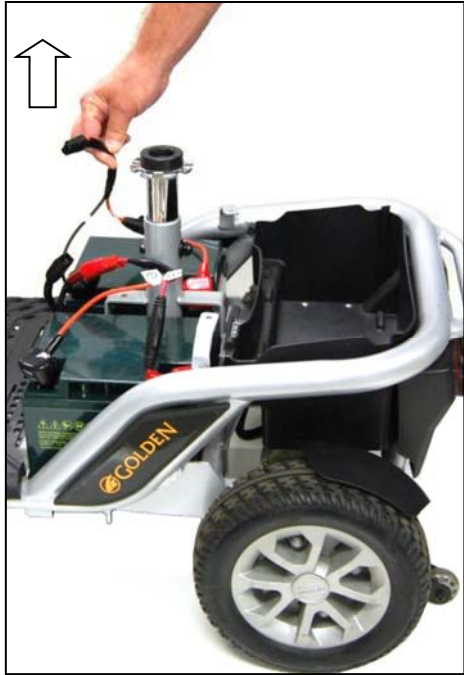
Figure 15. Removing Battery Cables
