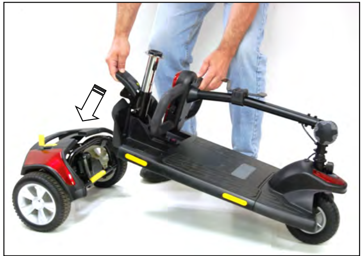
Figure 20. Connecting Frame and Drivetrain
