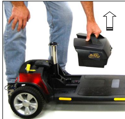
Figure 15. Removing the Battery Pack
