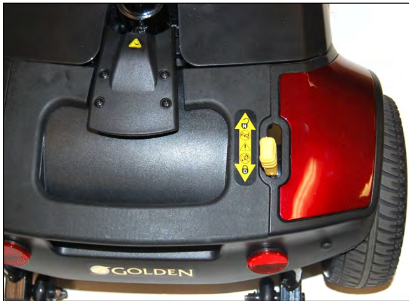
Figure 11: Freewheel Lever (Drive Position)
