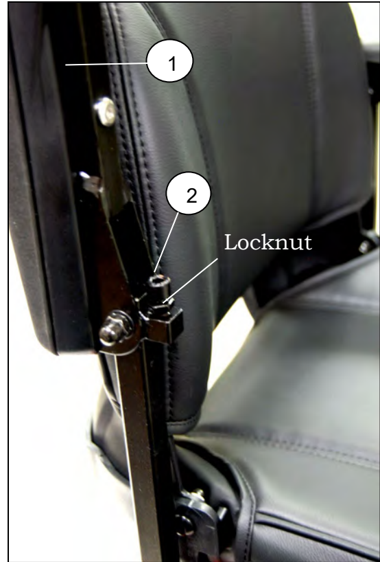
Figure 7. Armrest Angle Adjustment
