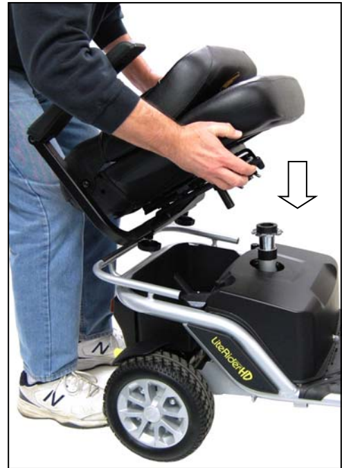
Figure 23. Installing the Seat
