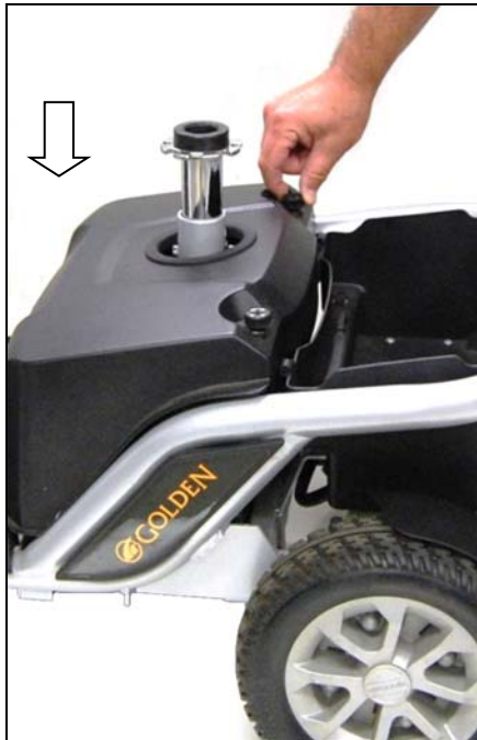
Figure 22. Installing Battery Cover
