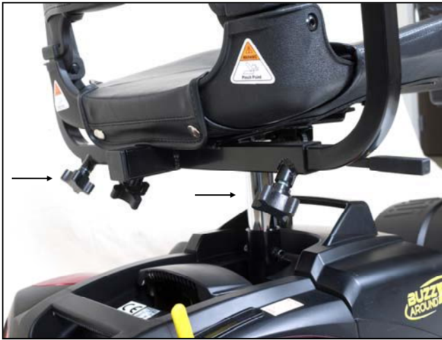
Figure 6. Armrest Width Adjustment
